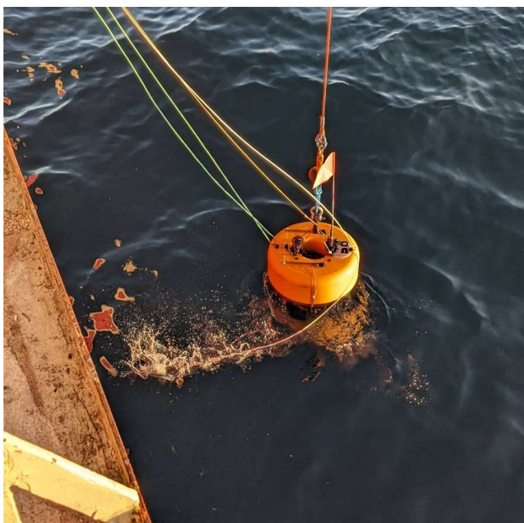
Figure 3-6: Aquarius OBS near water level about to be released. Note the high angle of the taglines and release pull rope. Total height from the water line to the winch deck is approximately 7 meters.
