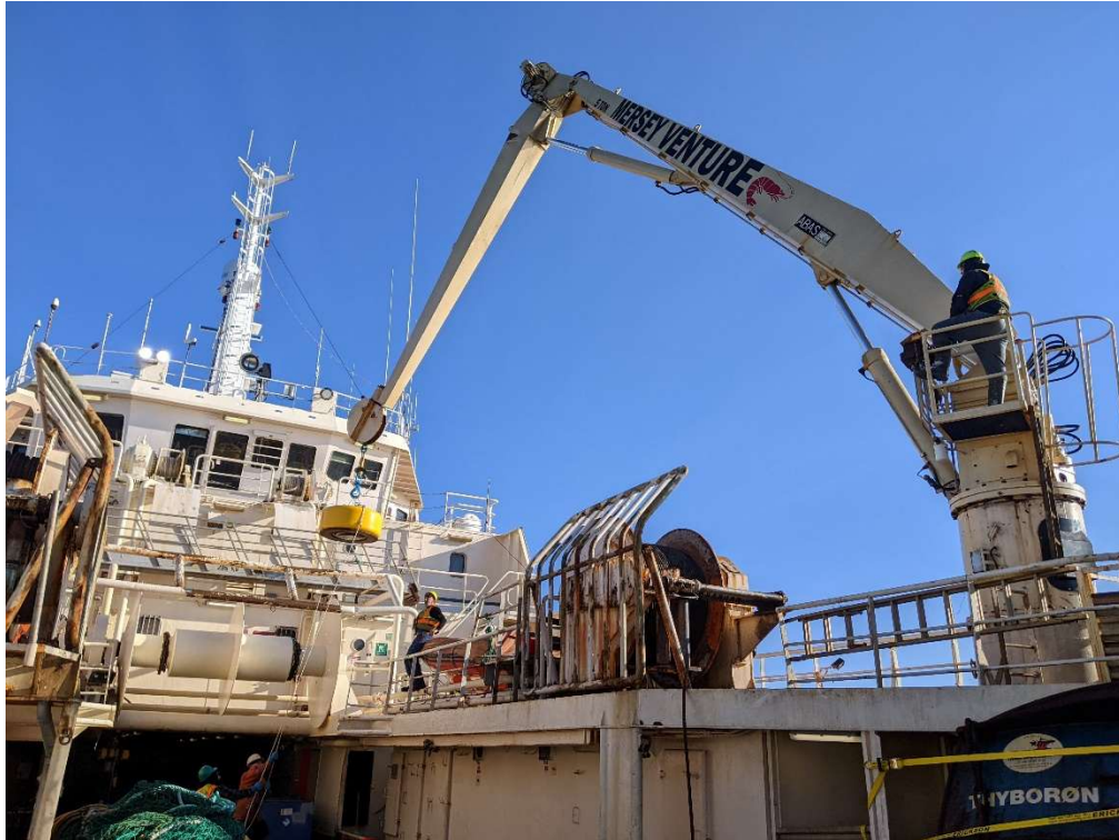
Figure 3-4: Lifting an Aquarius OBS from the trawl deck storage area to the staging area on the winch deck. Taglines were secured to either side of the buoyancy to control swing and passed up to the deck above as the lift progressed.
