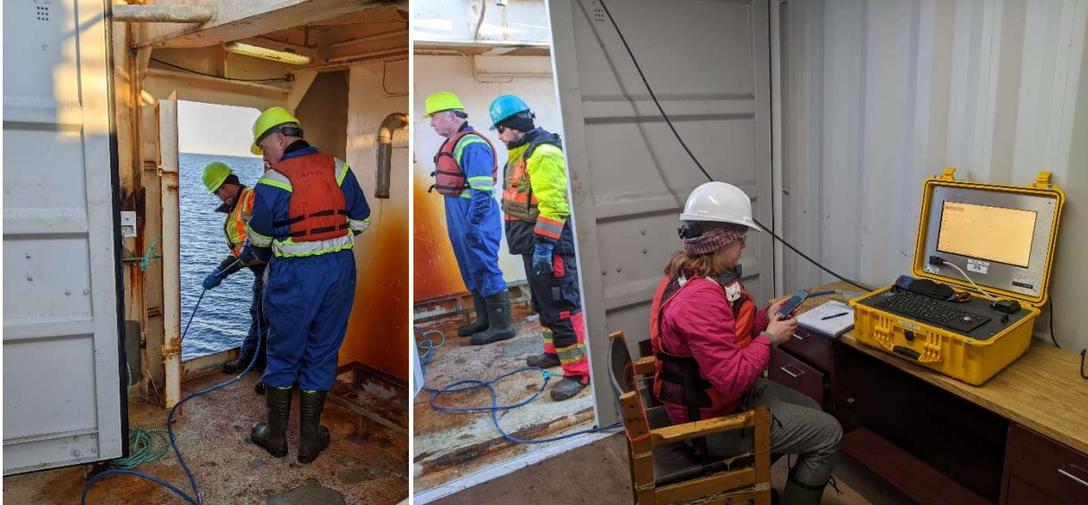
Figure 3-7: Dunker setup for in-water acoustic communication: (left) deckhands lowering the dunker on its cable through the door in the port side of the trawl deck, and (right) deck unit and NFSI technician Katie in powered container.
