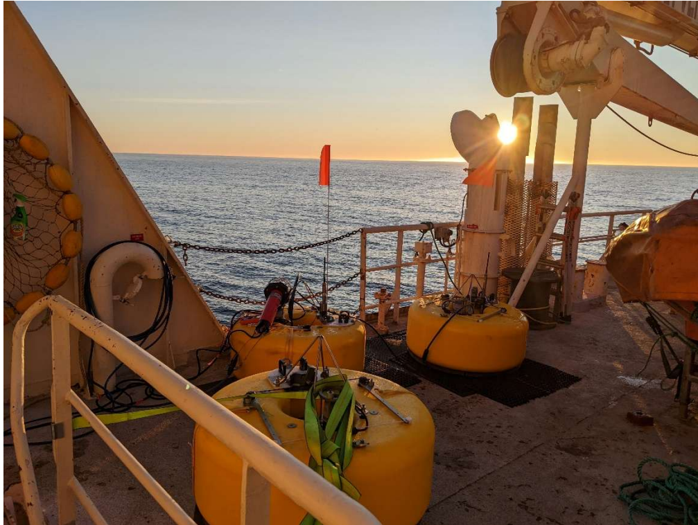
Figure 3-3: OBS staging area on starboard side of winch deck ahead of crane. Maximum of three Aquarius can be placed in this area and still allow unhindered foot traffic.
