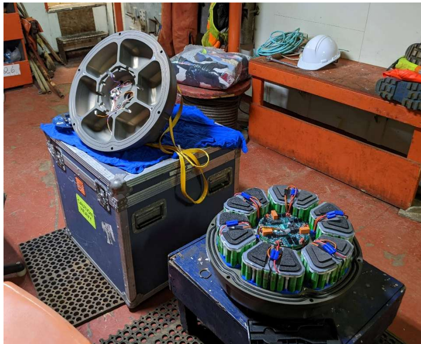
Figure 3-9: Aquarius OBS pressure case opened for repairs. All required maintenance was performed on the upper portion of the pressure case, which is tipped up at left.
