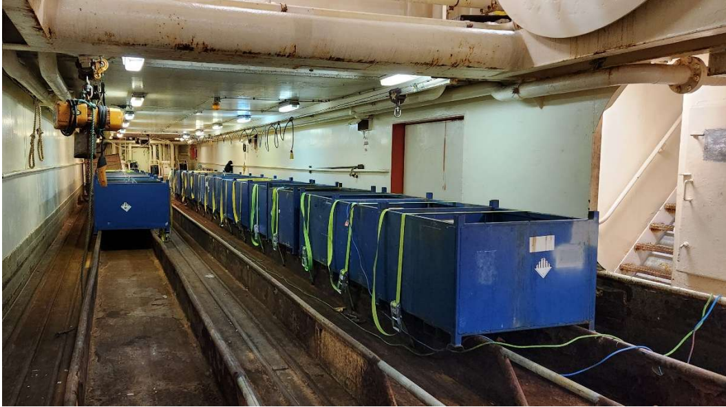
Figure 3-1: Aquarius stillage boxes stowed forward on trawl deck. The box legs straddle two adjacent rails, providing some lateral constraint on movement, and slide relatively easily out from under cover to move instruments to the staging area. Extension cords can be run out from the workshop for power as needed (blue and green cables at lower right).
